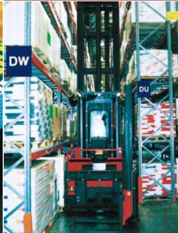
Above: Four Linde turret trucks provide fast cycle times in the very narrow aisle section of PaperlinX's Chullora DC.
