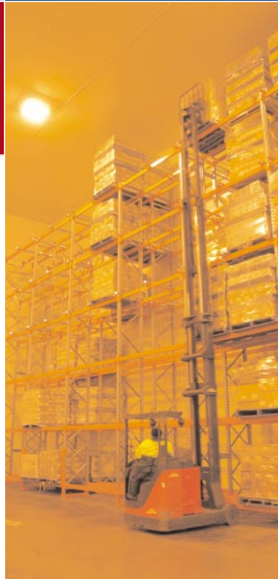
Above: A Linde Reach Truck stacking pallets at 10 m on double-deep racking.
