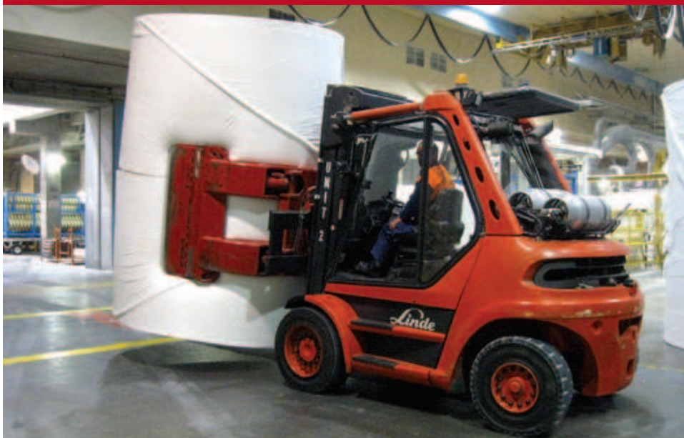
The Linde trucks used at SCA are fitted with very specific purpose-built attachments
